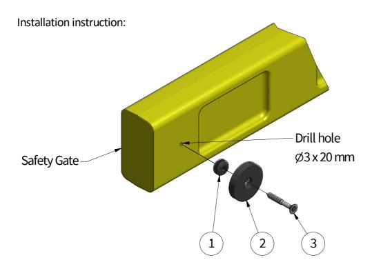
Tighten the screw so far that there is about 5 mm space between the magnet and the safety bar. The rubber washer is provided to secure the magnetic disk, but still allow the disk to be free to "float" or "wobble". In this way, the magnetic disk can make good flat contact with the metal guardrail post.
