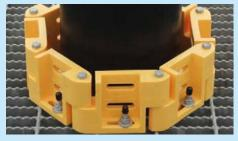
Once all the J-bolts are securely fastened, tighten each of the ¾" x 3 ½" bolts in the connecting holes.
