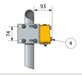
Supplied with U-bolts suitable for 42-48 mm pipe. All steel parts are galvanized.
