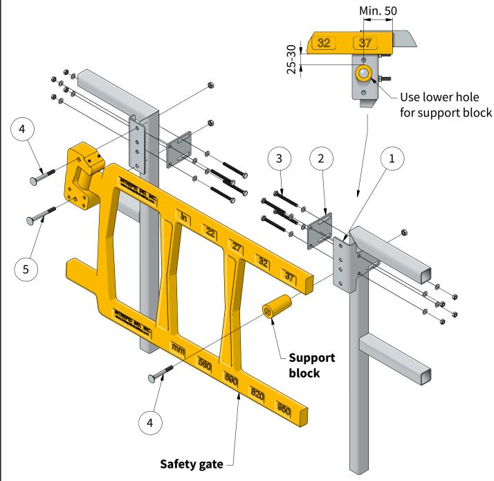
Fits on tubes 30-70 mm. Bolts for 80 mm tube on request.
