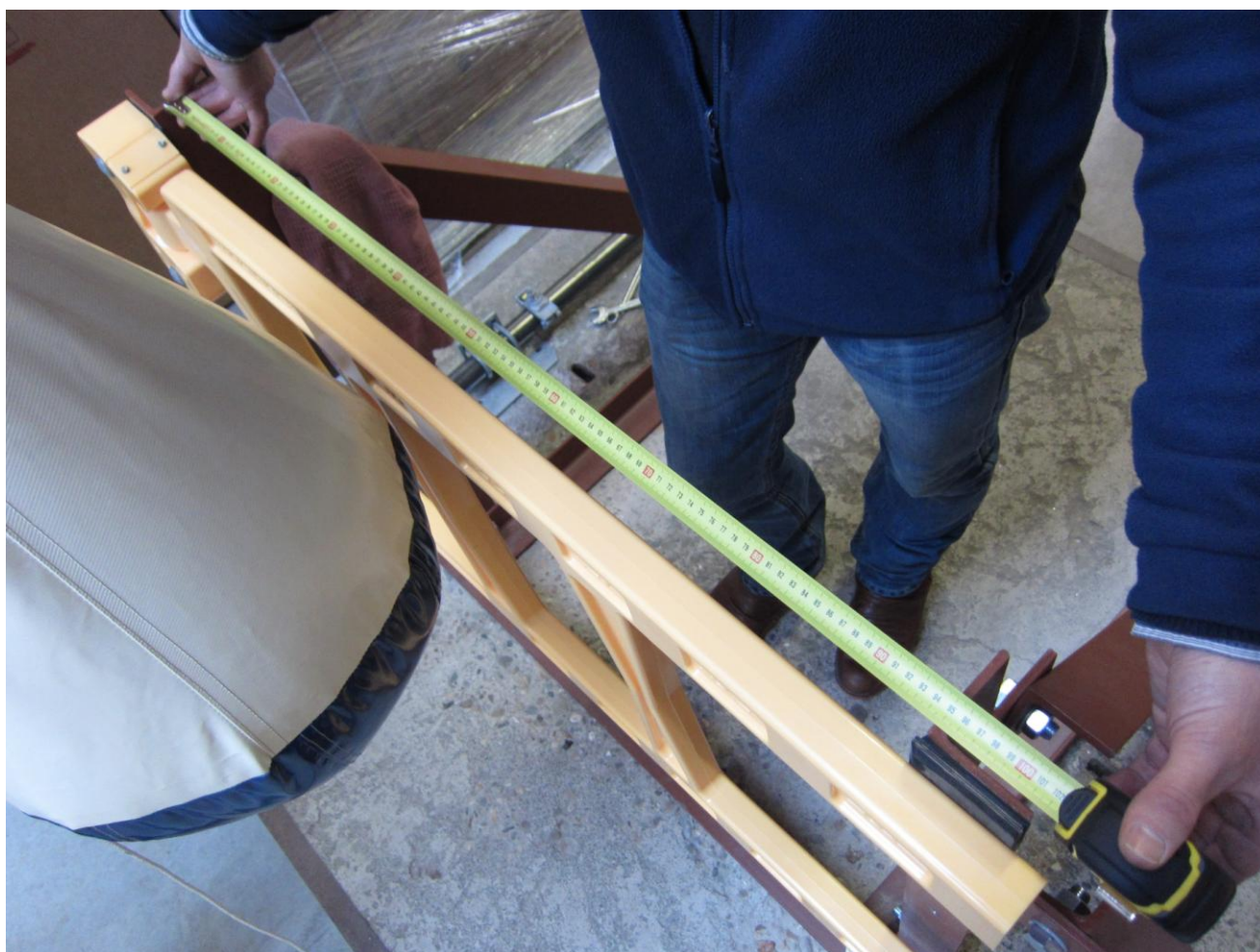
Photo 1, overview of impactor, frame, test specimen, measurement of width between L2's (95 cm)
